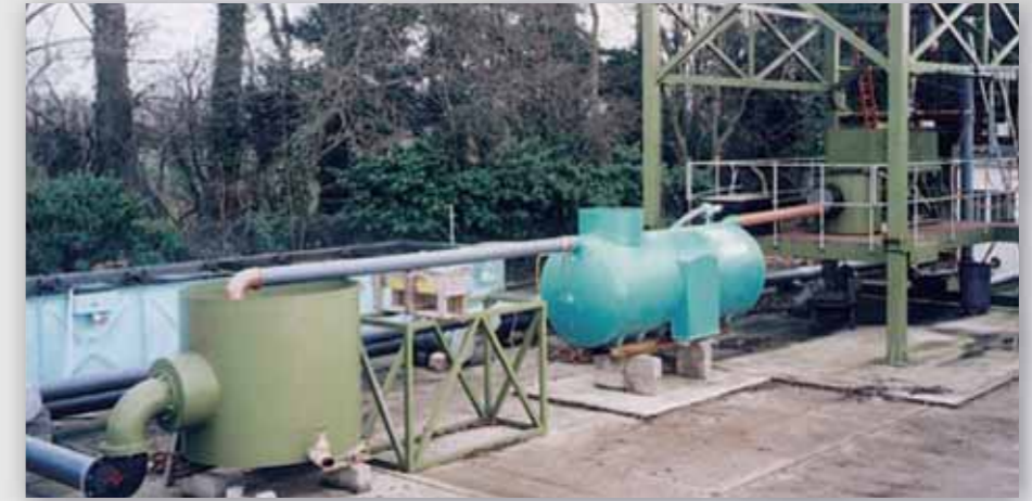
SPEL PURACEPTOR™ undergoing tests at HR Wallingford in accordance with European Standard BS EN 858.1. 2006
